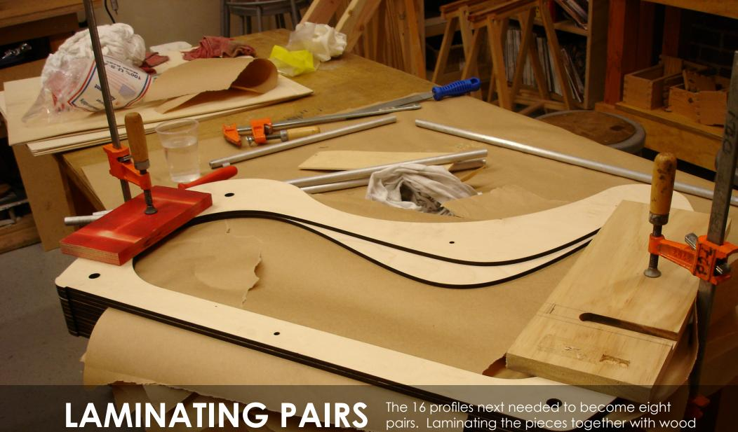
pairs. Laminating the pieces together with wood glue increased their overall strength and especially their resistance to bending. It also gave me two edges per section to support the foam on the stepped feature below the seat.
