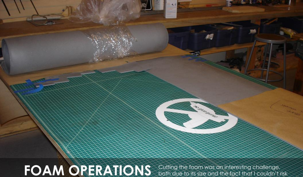
both due to its size and the fact that I couldn't risk leaving any marks on it. I used a combination of blue masking tape and butcher paper to guide my cuts. A gigantic piece of aluminum bar stock served as an eight-foot straight edge.
